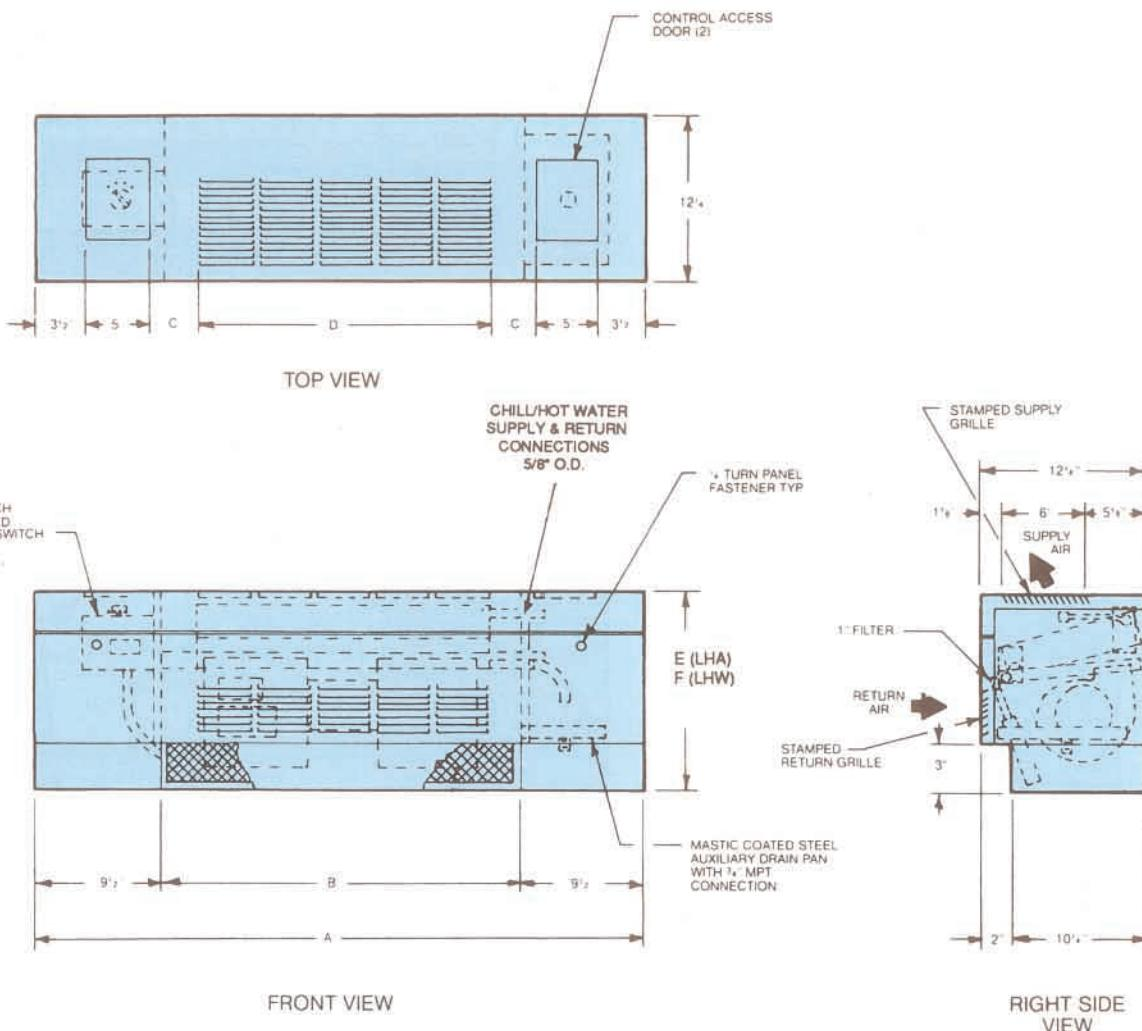
"Tall" Cabinet is used for applications w/electric heat. Cabinet is 2" taller than standard cabinet. Contact Factory for specific dimensions and drawing.
