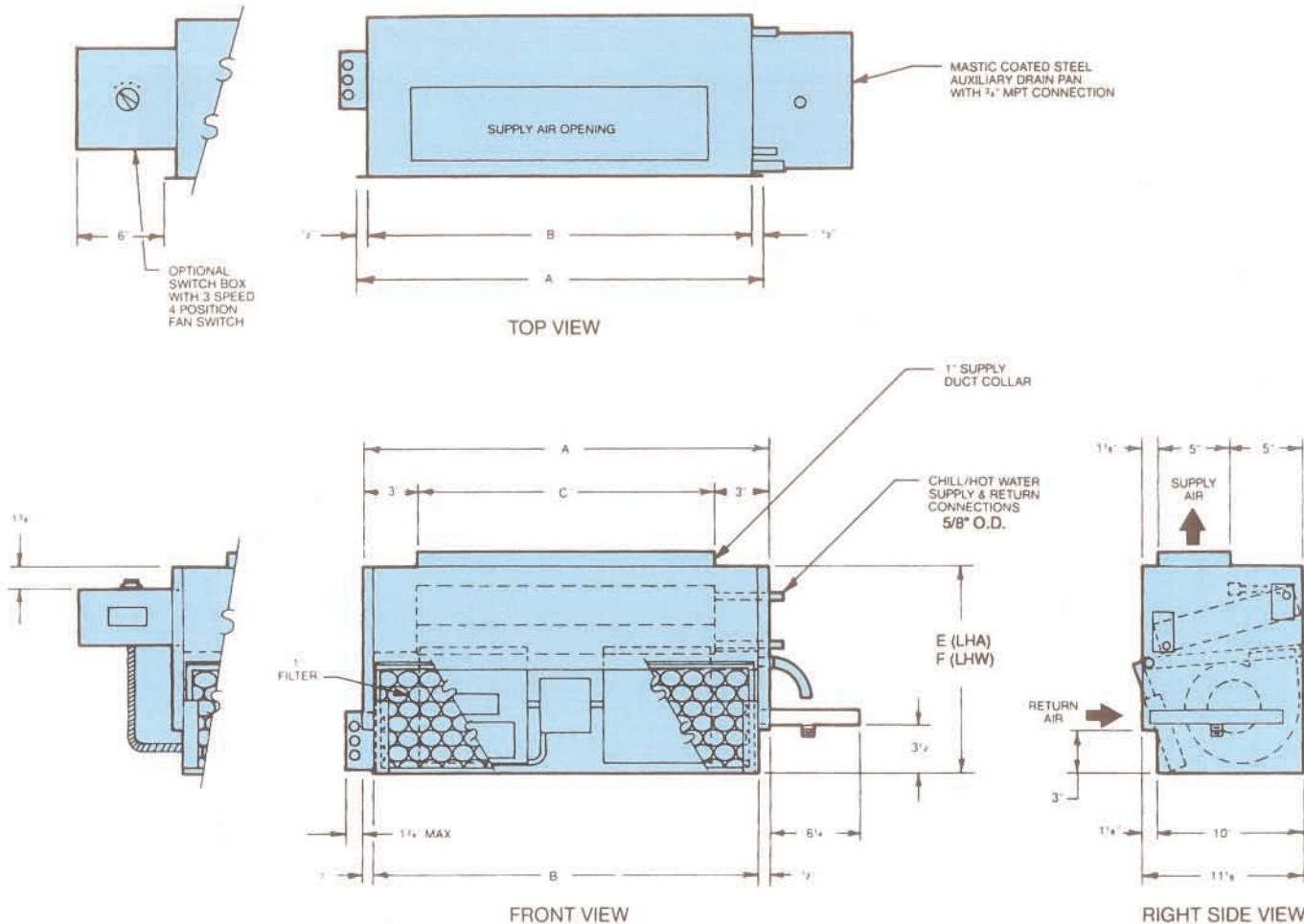
"Tall" Cabinet is used for applications w/electric heat. Cabinet is 2" taller than standard cabinet. Contact Factory for specific dimensions and drawing.
