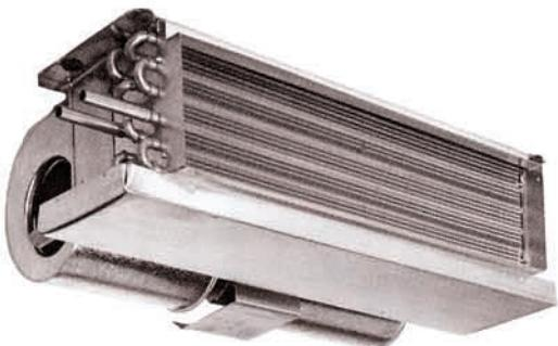
The model HBS Horizontal Fan Coil Unit is designed specifically to meet the many varied requirements demanded of the concealed type installation. The versatility of application and the low silhouette styling makes this unit ideally suited to drop-ceiling or over-closet applications. The design of the unit provides a positive pitch to drain when the unit is installed level, assuring rapid and positive condensate removal. HBS is provided standard with a galvanized finish.
