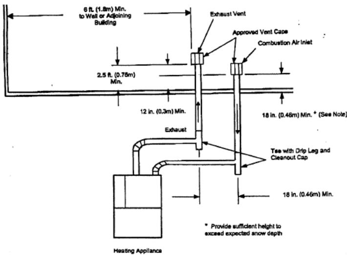
Figure 4 Separated Combustion Horizontal Venting
